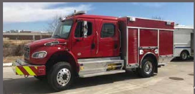
A new four wheel drive wildland-urban interface engine has been delivered to LFRA. The new engine is designed to fight wildland and structure fires in the rural areas of our response district. It carries 500 gallons of water and can pump 1000 gallons of water per minute. The new engine will be housed at Fire Station 2 once it is ready for service. This engine replaces a 1992 engine that served at Station 8 in Drake.
