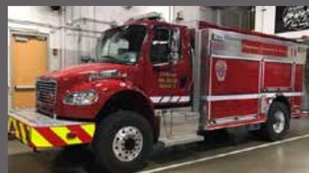
LFRA placed three new water tenders in service in January. The tenders were built by Rosenbauer Fire Apparatus on Freightliner 4X4 cab and chassis. Each tender carries 2000 gallons of water and has a 500 gallon per minute pump on board. The water tenders respond to fires in rural areas that do not have fire hydrants, the tenders supply the fire engines with the needed water for firefighting operations. The new tenders are assigned to Stations 3, 5 and 8, replacing twenty one year old tenders.
